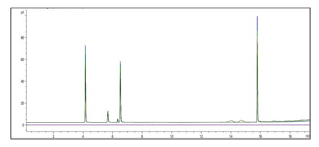
The chromatogram showed that there was no time shift after repeated injections, which means the results should be consistent and the lifetime was not significantly reduced even if the samples contained some "active" components.
