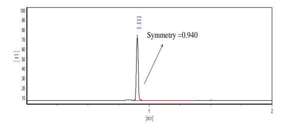
In the second part, ethanol separation was achieved on 2632-3002. Ethanol, methanol, acetone and acetic acid are not easily extracted from aqueous samples and the demand of such component analysis is highly increased, especially in liquor industry. Therefore, we provided the solvent analysis results with repeatability test.
